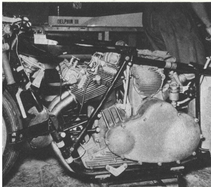
Supercharged power plant used by NSU for record runs develops 110 horsepower. Only eight of its kind exist.
