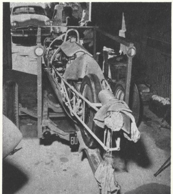
Mangham's machine uses mass-produced engine, gets record speed from radical design. Parachutes are for braking.
